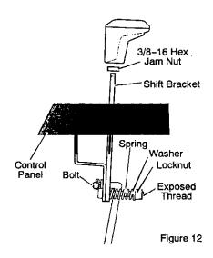
3. Tighten the 3/8–16" hex jam nut against the knob securely.
